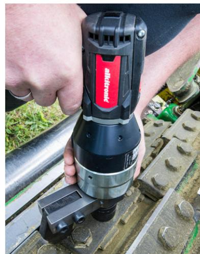
Repeat shut-off accuracy ± 3% (same bolting connection). All **alkitronic®** torque multipliers are CE-certified.
