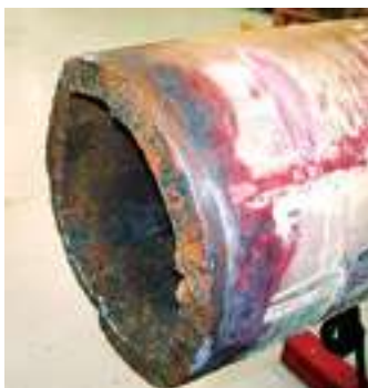
Hot torch cut before machining
