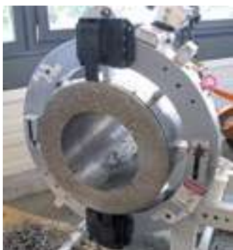
LCSF with worm slide assembly
