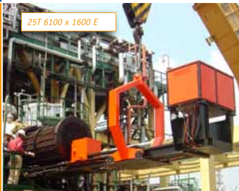
25T extractor with 30T combi lifter
